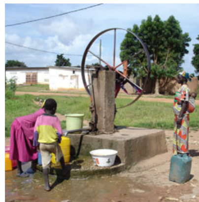
Volanta pump in use in Cameroon
