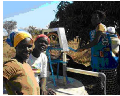
rope pump in use
