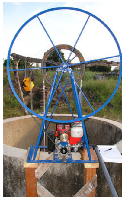
the motor rope pump on an open well
