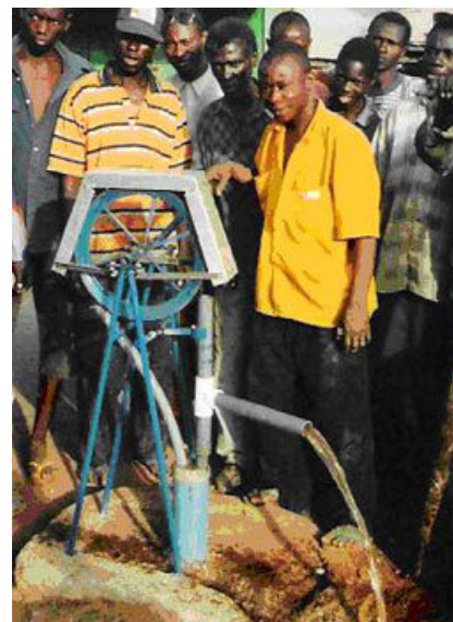
rope pump installed on a bore hole
