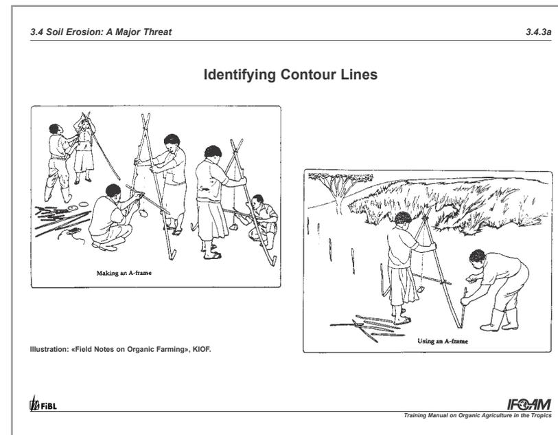
*Transparency 3.4.3a: Building and using an A-frame for identifying contour lines (source: "Field Notes on Organic Farming", KIOF).*
