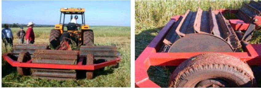
The Knife Roller to flatten and kill green manure cover crops and leave the plant residues on the soil surface is an essential tool for cover crop management.
