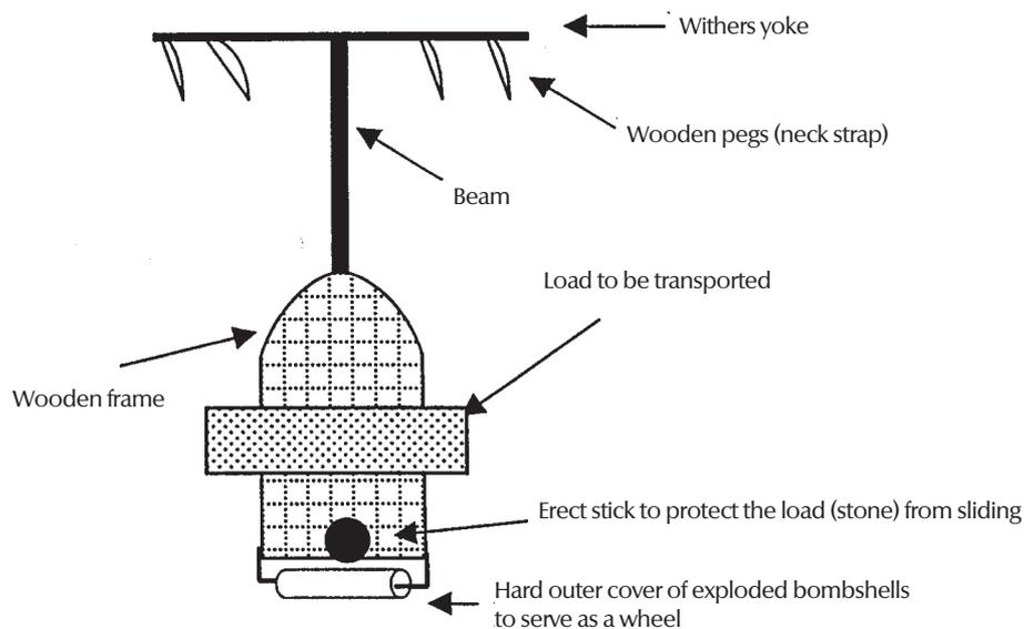
Figure 1. Menkorkor used to transport heavy loads
