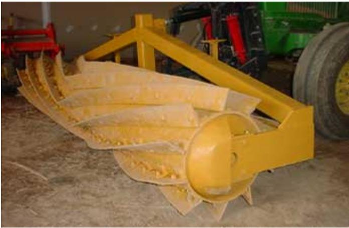
**The Rodale Institute® Farm Manager Jeff Moyer reports** the front-mounted three-point hitch with a hydraulic lift was easy to bolt on to the factory frame openings. It was a medium price-range product with limited mobility, making lining up the hitch with the roller a bit challenging. But, it worked well for the roller. Now that he has the hitch, Moyer and crew are looking for other uses, such as adding a cultivator toolbar or skid forks.
