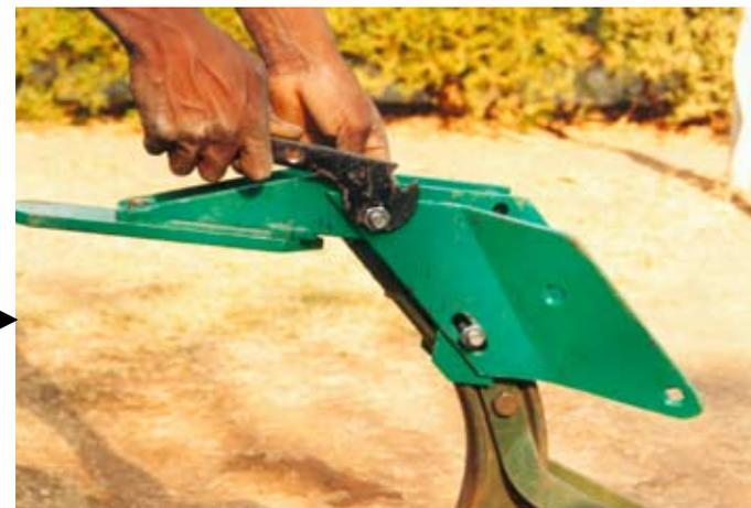
Attaching the **sub-wings** to the ripper tine body. Always use the correct size spanner for the job! The tine is reversible when it gets worn.
