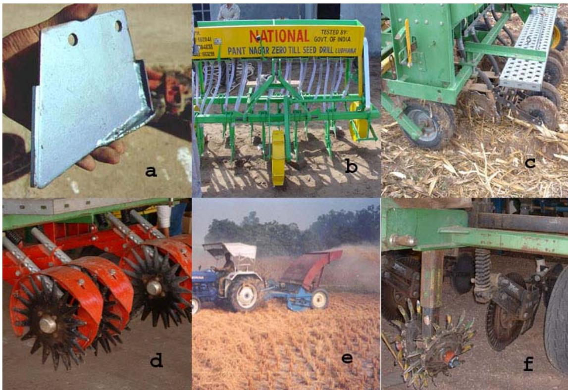
**Figure 5. Various equipment for planting wheat no-till in the RWC: (a) inverted-T coulters; (b) Indian no-till drill using inverted T; (c) disk type planter; (d) star-wheel punch planter (e) “Happy planter,” which picks up straw and blows it behind the seeder; f) disk planter with trash mover.**
