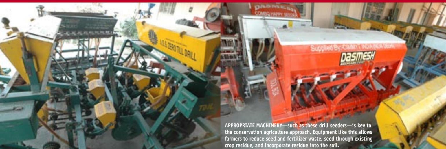
APPROPRIATE MACHINERY—such as these drill seeders—is key to the conservation agriculture approach. Equipment like this allows farmers to reduce seed and fertilizer waste, seed through existing crop residue, and incorporate residue into the soil.
