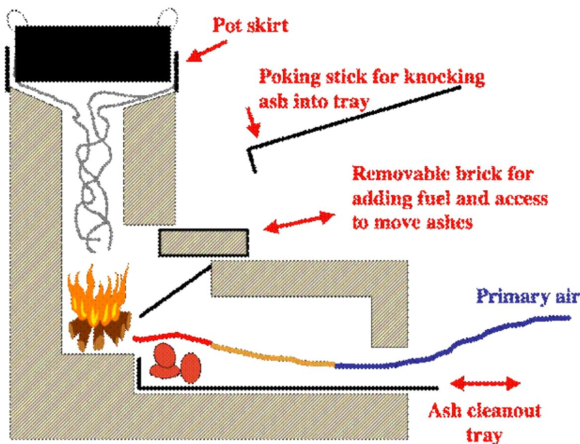
Figure 10: Concept Schematic of Weyer's Prototype Stove
