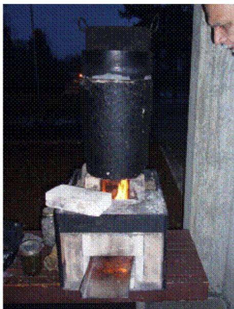
*Figure 11: Weyer Dung-Burning Prototype Stove*
