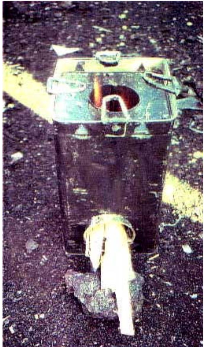
**Efficiency:** 12-42%. The efficiency depends on type of a heat exchanger used.
