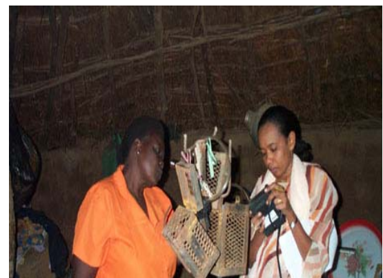
Monitoring for smoke – the monitors are housed in metal boxes for safety (photo: ITDG)
