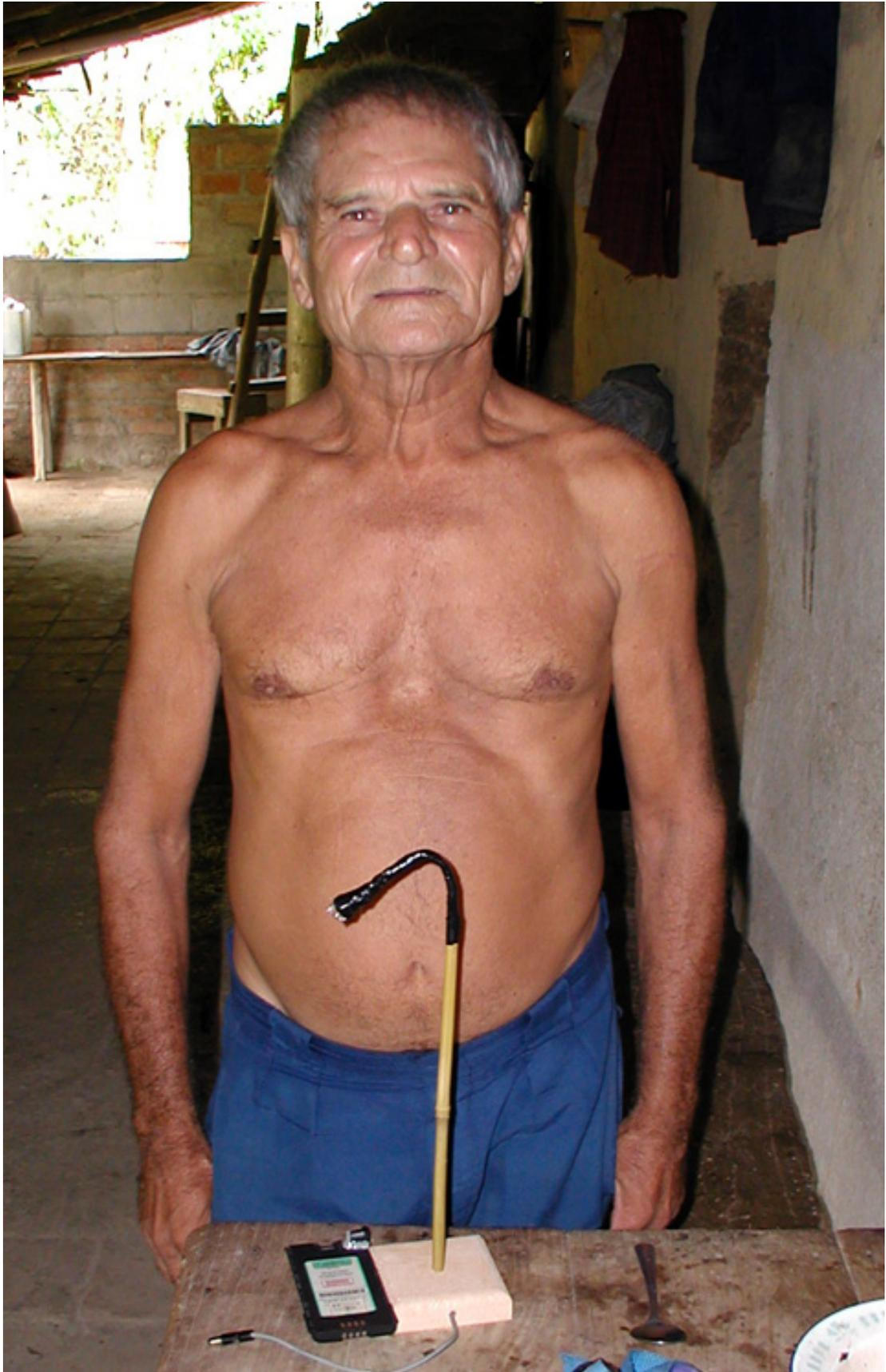
This is an LED light with five bulbs and a Motorola six-volt cell phone rechargeable battery.
