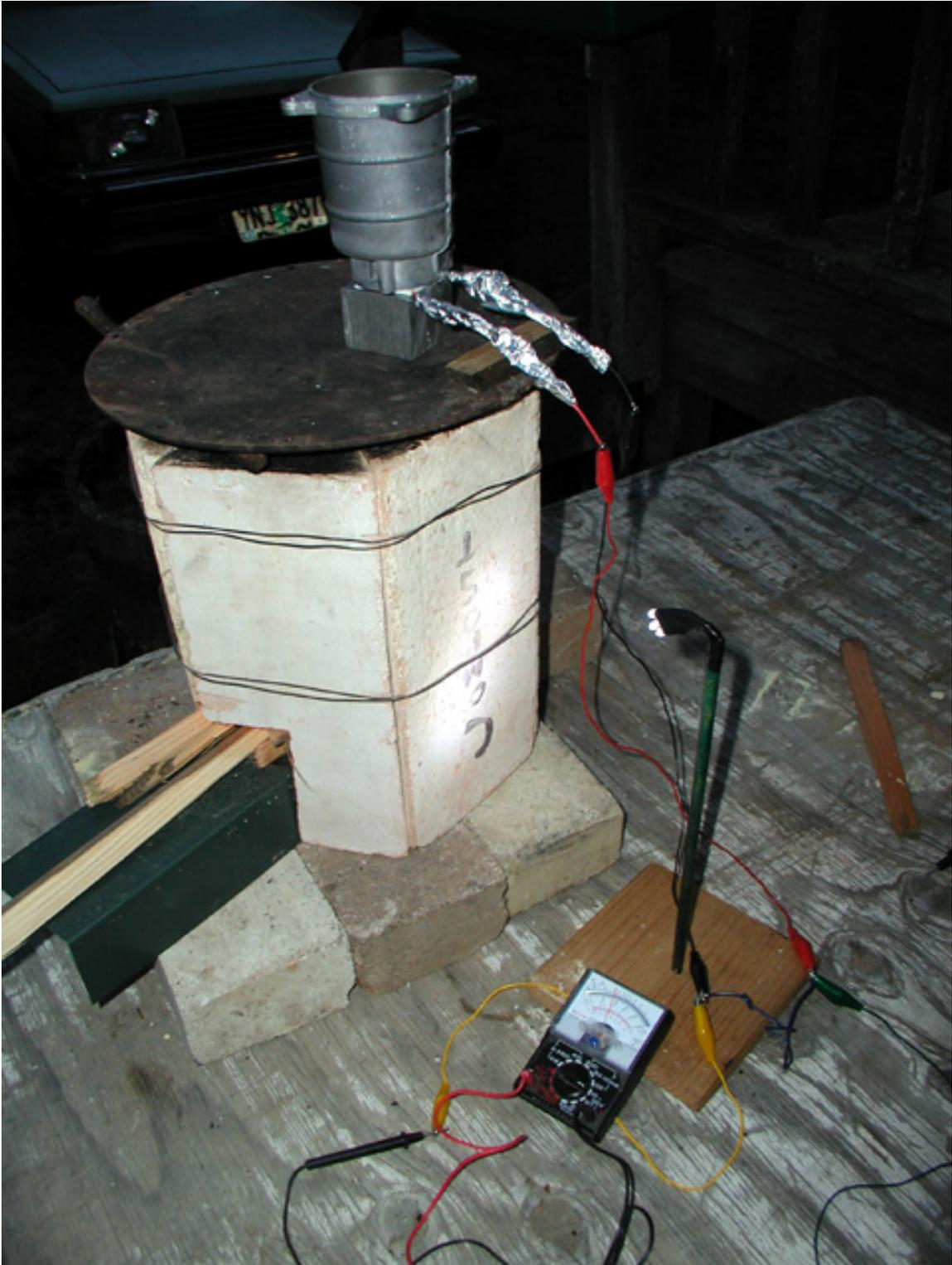
This is a three bulb LED light running from a single thermocouple powered by a six brick stove.
