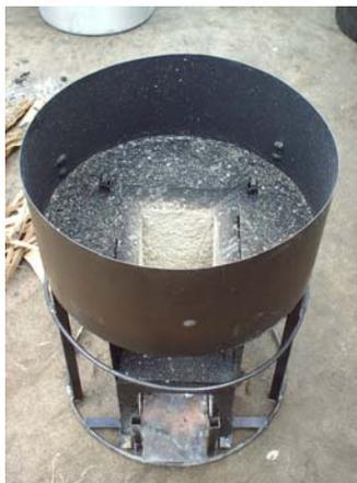
differences. First, the stove is cheaper and easier to build and second, it features an insulated top plate. This top plate has two features: it improves heat transfer into the pot and it increases the longevity of the stove, as there is less metal exposed to open flame. Although no lab tests were performed
