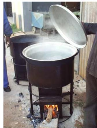
on the MangiMangi, an informal test showed that it could boil 40 Litres of water in 35 minutes with 2 kg of wood. Cooking tests as well as a WBT should be performed on the stove to ascertain its overall efficacy. Initial response from cooks at Formigas del futuro has been overwhelmingly positive.
