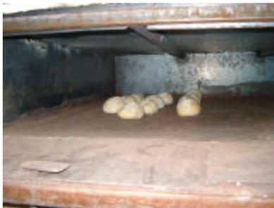
The rolls, which are cooked directly on clay tiles, require 300 degrees Celsius, as compared to 'loaf' type breads that require only 180 degrees Celsius. The 2mm sheet metal box (which has proved effective in Lesotho and Uganda) was not sturdy enough to withstand these higher temperatures. There were also other complaints such as uneven baking temperatures. The oven was too hot on the bottom and too cold on top.
