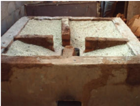
The third prototype was modified to incorporate 4 courses of bricks so as to offer more support to the baking compartment. The 4 corners of the outer structure were also reinforced with solid brick instead of thinner walled Ceramica Villa Pery building blocks.
