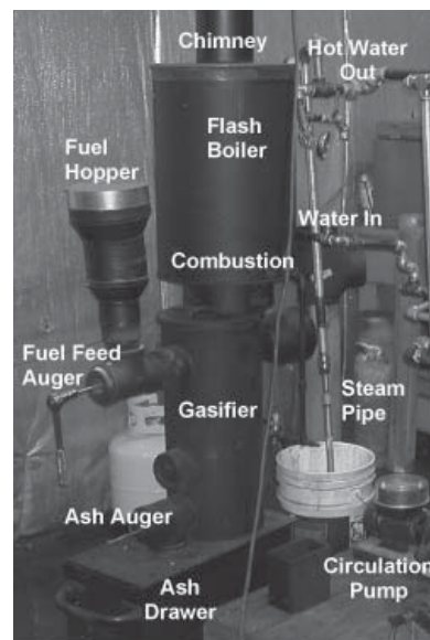
Figure 4 The AVUD gasifier is the lower vertical cylinder with its openings for fuel entry, ash removal, and air flows. Left is the open-cart version of the Chip Energy Biomass Grill (US$150) with the combustor in the tray under the plancha griddle top, plus the chimney. The cart is essentially “stove structure” that could be adobe blocks or stainless steel walls. Right is the Chip Energy Furnace for process heat (200,000 BTU = 211 megaJoules = 50,400 kcal) with combustion at the center of the picture and a flash boiler application in the upper cylinder. Other applications of process heat are easily adapted. (photos: Chip Energy)
