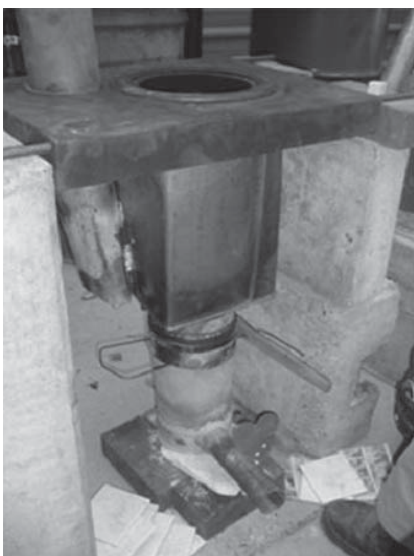
Figure 3 Examples and explanation of natural draft TLUD stoves. Left is the 2005 Champion stove. Right is the Andreatta TLUD testing device of 2007. (photos: Paul Anderson, left and centre, Dale Andreatta, right)
