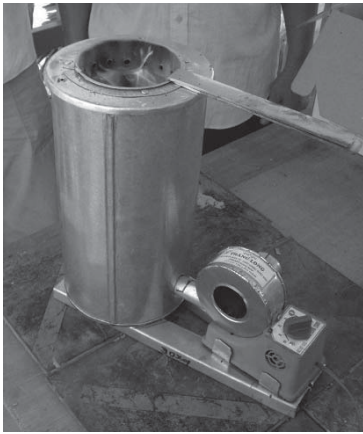
Figure 2 Reed's Woodgas Campstove (left) for sale on the Internet (US$55) and Anderson's Juntos B+ TLUD gasifier (with removable fuel canister) hand-made in Cambodia with GERES (estimated cost under US$20). For cooking, the pot can be placed on top of the unit or (better) be positioned on a simple pot support structure of any size so that the gasifier can be moved for refilling without disturbing the pot. (photos: Tom Reed, left, Paul Anderson, right)
