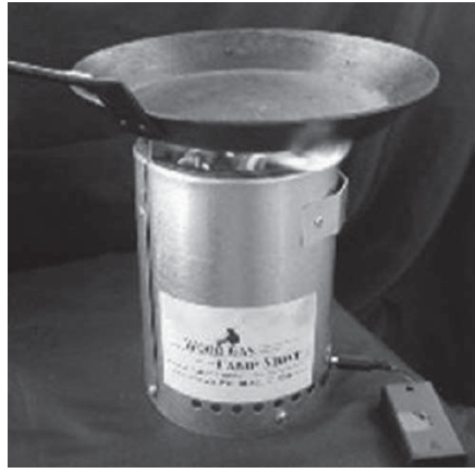
Figure 2 Reed's Woodgas Campstove (left) for sale on the Internet (US$55) and Anderson's Juntos B+ TLUD gasifier (with removable fuel canister) hand-made in Cambodia with GERES (estimated cost under US$20). For cooking, the pot can be placed on top of the unit or (better) be positioned on a simple pot support structure of any size so that the gasifier can be moved for refilling without disturbing the pot. (photos: Tom Reed, left, Paul Anderson, right)
