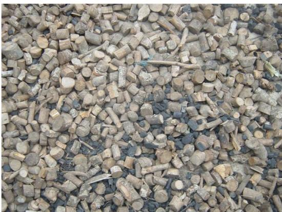
**Photo G3: The chips from the waste wood and bamboo that will be the feedstock for the gasifier**
