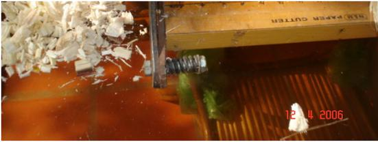
**Photo G5:** Sugar cane bagasse after chopping with a guillotine. A way has to be found to mechanize this process and still achieve the necessary reduction in size
