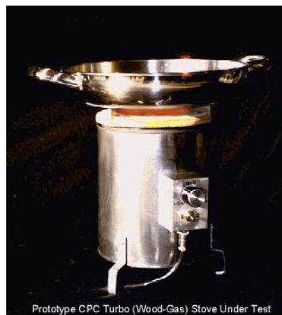
Figure 8. Turbo Wood-gas Stove (Reed and Walt, 1998).
