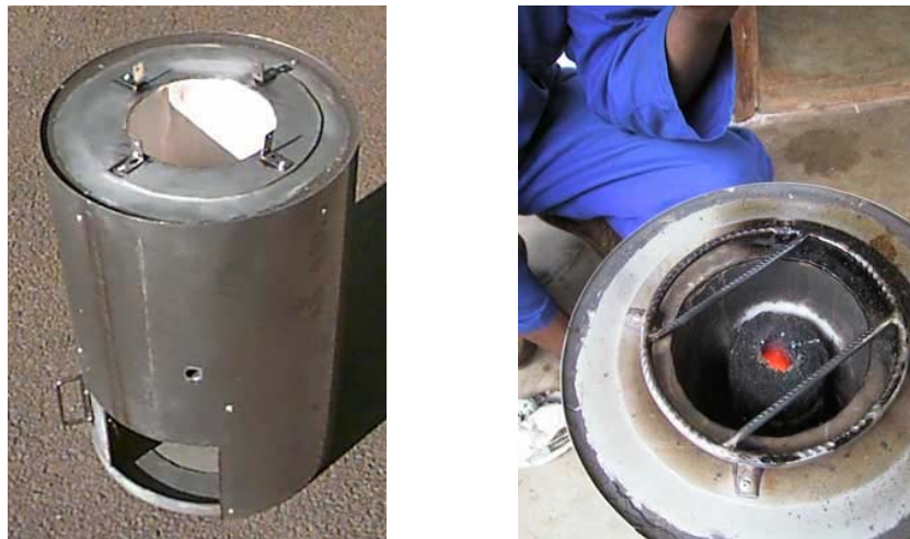
Prototype briquette gasifying stove
