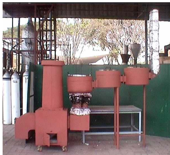
Figure 7: Commercial Gasifier Stove CGS3 developed at AIT (11.5 kW; 31% efficiency with woodchips)
