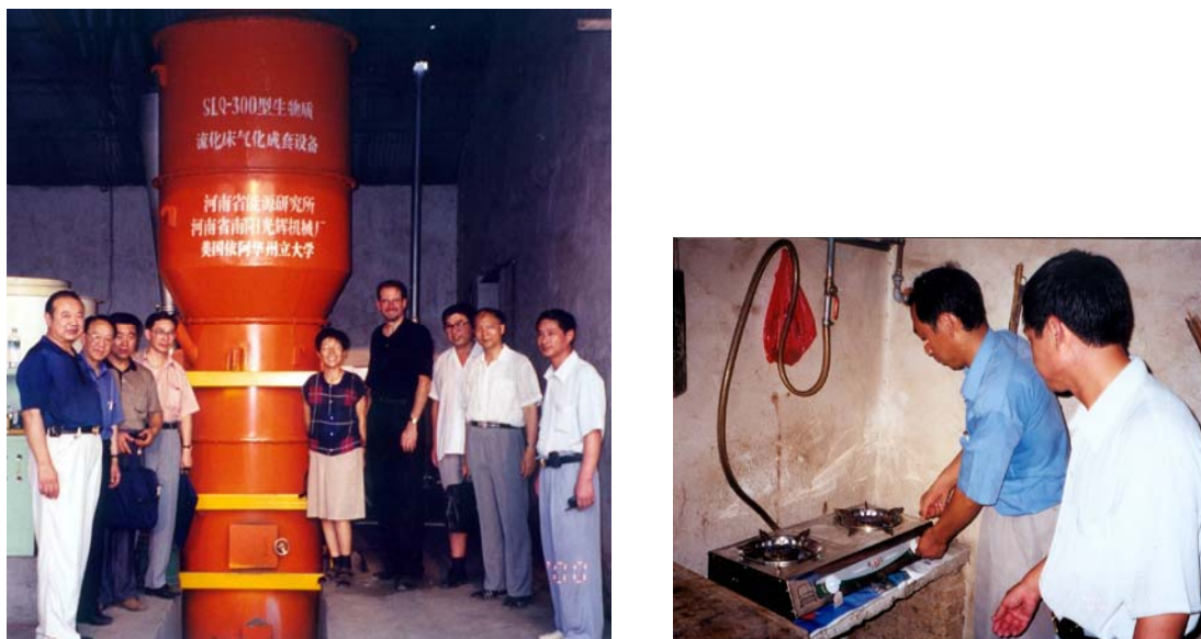
Figure 12: The Fluidised Bed Gasifier generating producer gas from peanut shells, developed in China
