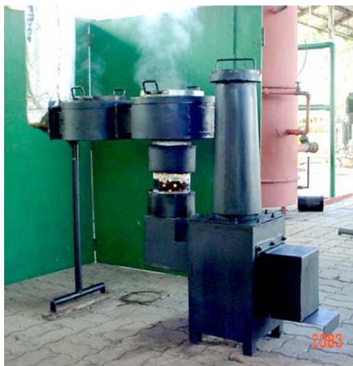
Figure 6: Institutional Gasifier Stove IGS2 developed at AIT (5.5 kW; 29% efficiency with woodchips)
