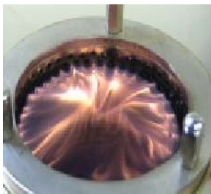
Figure 9. Flame inside the burner of the Turbo Wood-gas Stove
