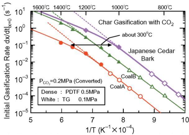
**Fig.1** Results of char gasification rate analysis of cedar bark
