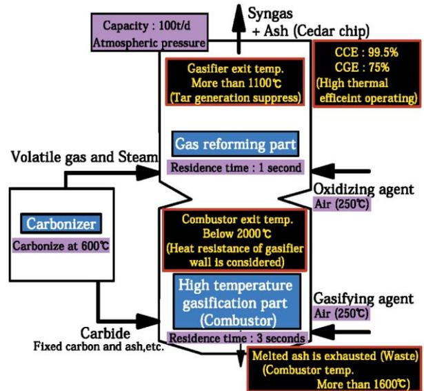
**Fig.2** Schematic of carbonization and gasification system
