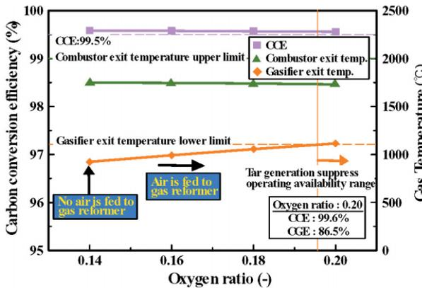
**Fig.3** Gasification performance in carbonization and gasification system (Cedar chip, Combustor oxygen ratio = 0.56, Air is fed to gas reformer)
