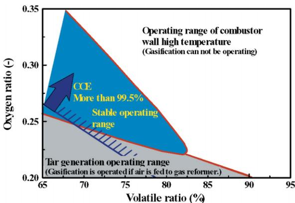
**Fig.5** Operating condition range for high thermal efficiency and stability when volatile ratio is changed.
