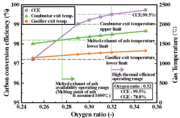
**Fig.4** Gasification performance in case of Waste
