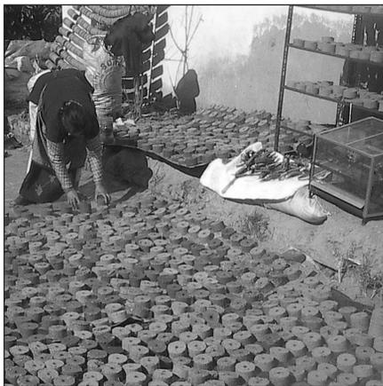
Figure 2 Environmentally friendly drying of briquettes (photo: FoST)
