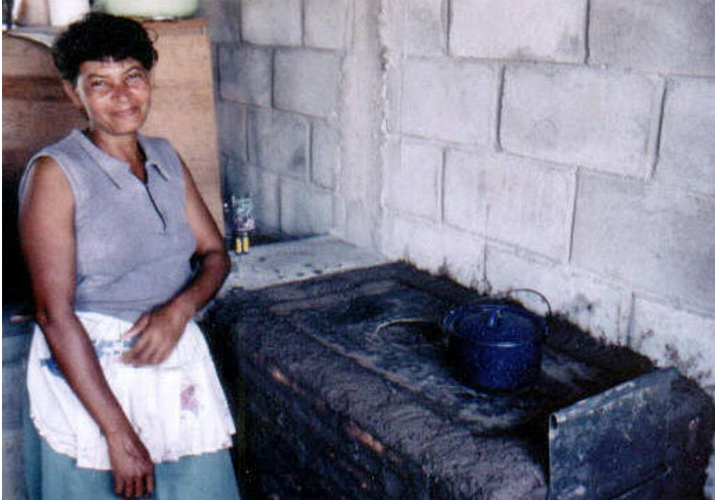
**Efficiency**: almost twice as efficient as an open fire when used with three pots. Insulated low-mass rocket combustion chamber reaches near complete combustion so wood is burned more effectively.
