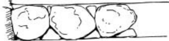
Figure 3: Uneven boulders need to be pinned
