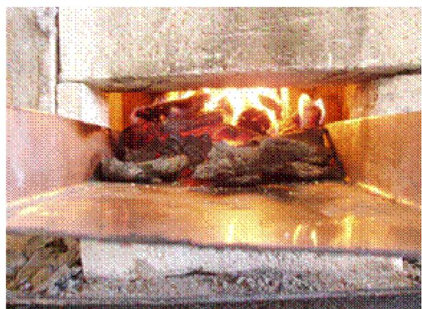
*Figure 14: Prototype Ash Tray*
