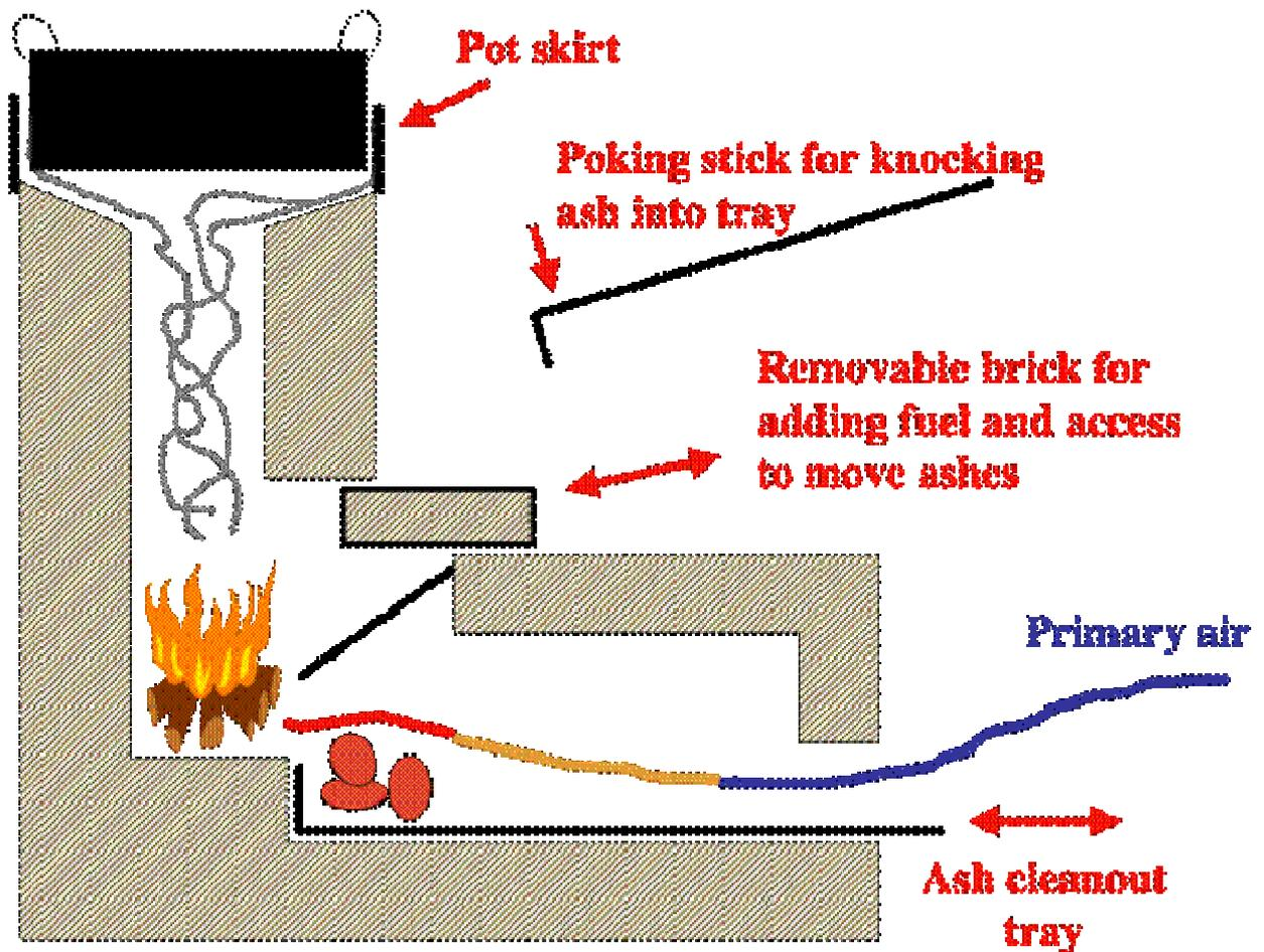
*Figure 10: Concept Schematic of Weyer's Prototype Stove*
