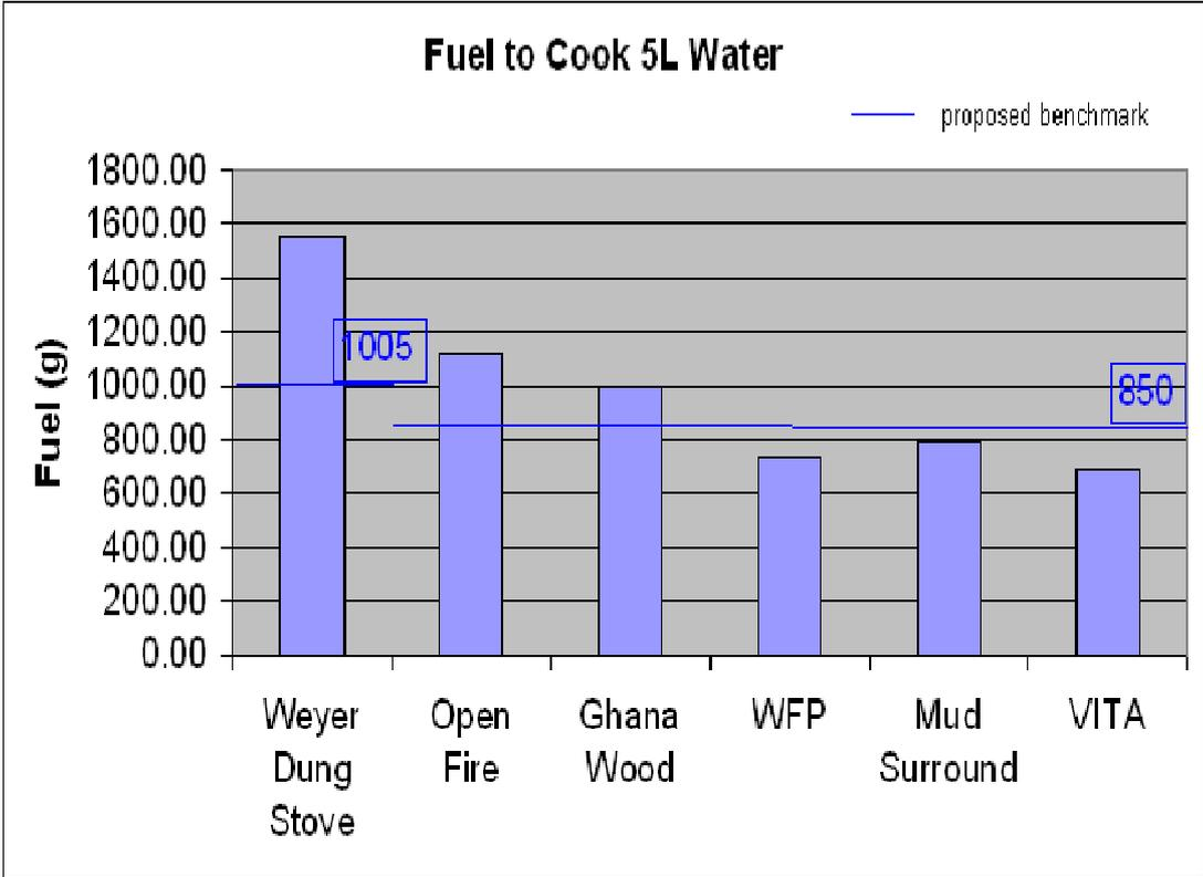
Figure 15: Comparison of dung stove to wood-fueled stoves for fuel used.
