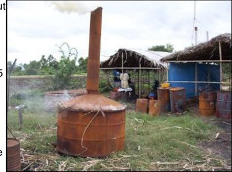
About 10 kg trash are burnt underneath the containers (in the kiln) to start the process of pyrolysis. The heat of the trash burning underneath the containers pyrolyses the trash in the container. Pyrolysis gas generated in the process leaves the containers through holes in their bottom, and it too burns, to serve as additional fuel in this process.
